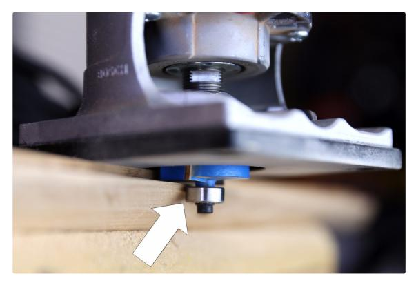
Set the router base to the depth desired, its always a good idea to run the router on a test piece of wood before committing to the project - that way you can make multiple adjustments if necessary. Carefully router every side until the edge profile desired is achieved.
