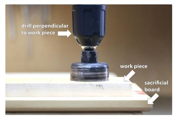
Even though hole saws are removing the perimeter of your hole and will create a plug when finished drilling all the way through, they are covering a lot of surface area and can get bogged down easily. Go slow with the hole saw and push gently, allowing the hole saw teeth to do the work.
