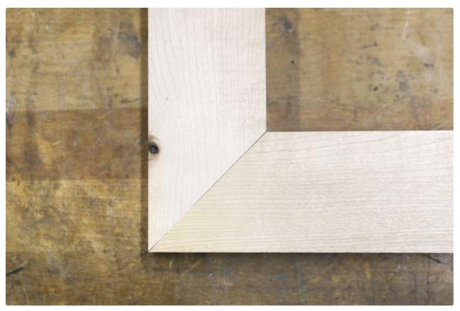
Up to now we've been focused on right angles with our wood projects, but there's going to be times when you're going to want more complex shapes to your woodworking. The next step to adding interesting details to your work is with angled cuts, in woodworking terms angled cuts are called either bevels or mitres.
