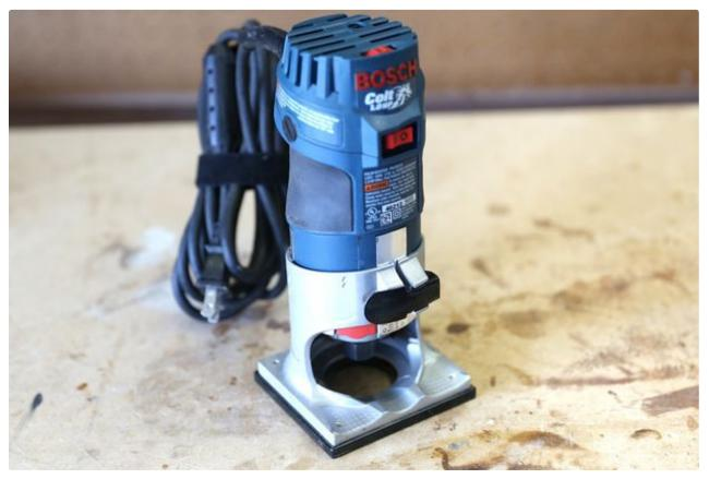
A hand router is one of the most versatile tools in woodworking. More than just a way to bevel an edge, a router can create all kinds of edge profiles, be used to square wood edges, and even used as a thickness planer to level uneven wood. In this lesson we'll be covering all those uses as well as breaking down the router to understand just how handy this humble tool can be.
