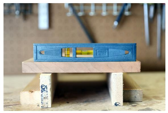
With both rails set up on your workbech a plank can be laid across the top of the rails to check if they are level. If there's any discrepancy check the workbench for levelness first, then check the rails to ensure they are symmetrical.
