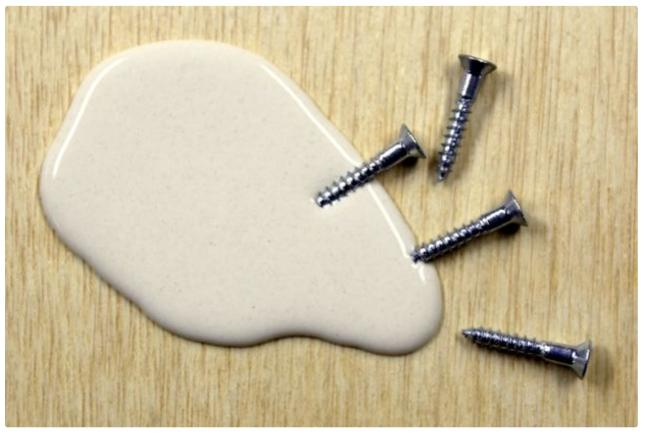
For woodworking there's a few types of glue that are used, but by far the most common is carpenter's glue. This type of glue is called polyvinyl acetate adhesive, or PVA for short. PVA glues are inexpensive and have great holding ability, making it an ideal woodworking adhesive.
