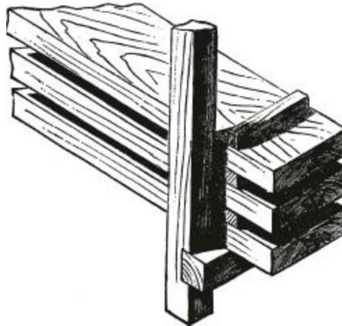
Fig. 505.—Timber Stacked on the Flat.
