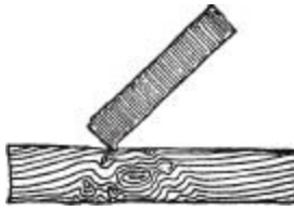
Fig. 424.—Using Badly Sharpened Scraper.
