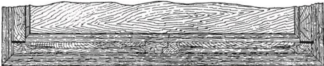
Fig. 2329.—Moulded Edge of Plate Cabinet Top.
