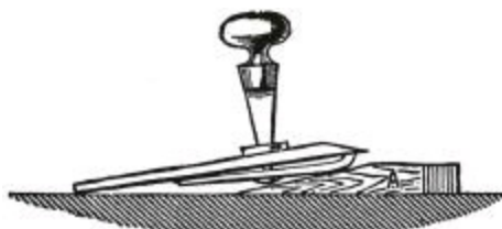
Fig. 163.—Unscrewing Plane Irons with Special Tools.
