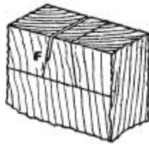
Fig. 683 —Saw Kerf in Waste Portion.
