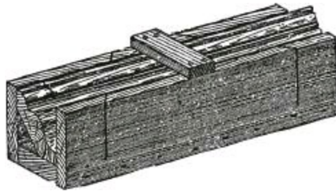
Fig. 59.—Mitre Box with Strengthening Piece.
