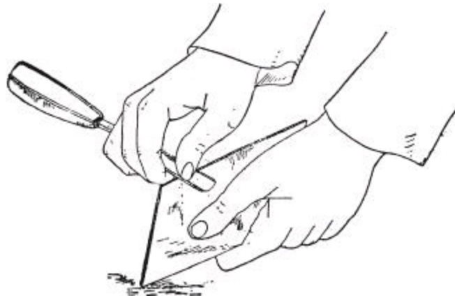
Fig. 422.—Forming Burr Edge on Scraper.
