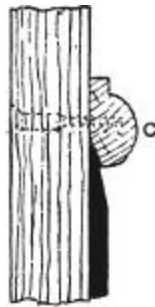
Fig. 2019.— Mirror fixed with Moulding.
