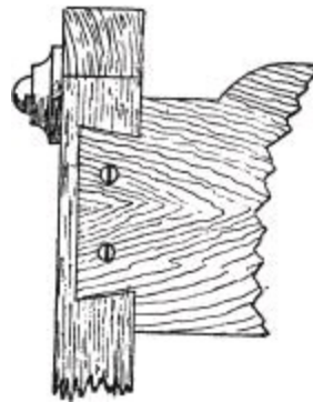
Fig. 1696.—Joint of Back to Side of Rack.
