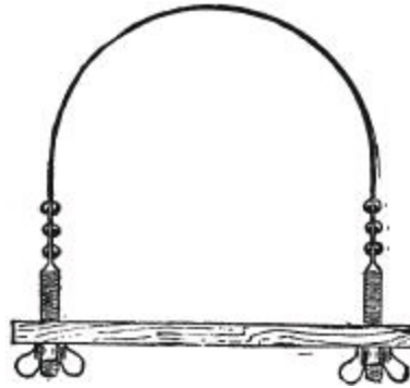
Fig. 126.—Screw-end Flexible Cramp.
