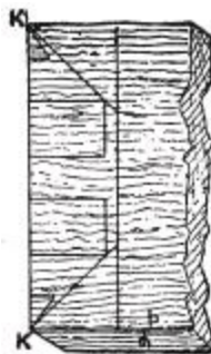
Fig. 652.—Setting Out Mitre Clamping.
