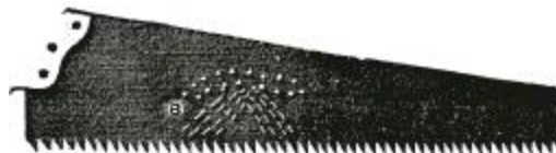
Fig. 319.—Buckled Hand Saw.
