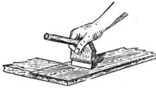
Fig. 1677.—Method of Using Veneering Hammer.
