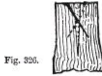
Figs. 326 and 327.—Fastening on Hammer Head with. Nailed Wedge.
