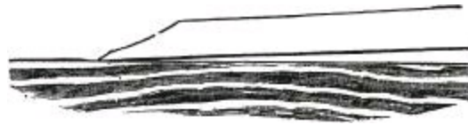
Fig. 145.—Badly Sharpened Chisel Edge.
