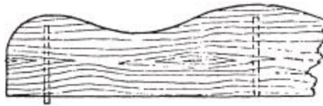
Fig. 2116.—Mantelboard Stiffened with Metal Tubing.
