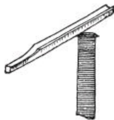
Fig. 423.—Wrong Method of Forming Burr Edge.
