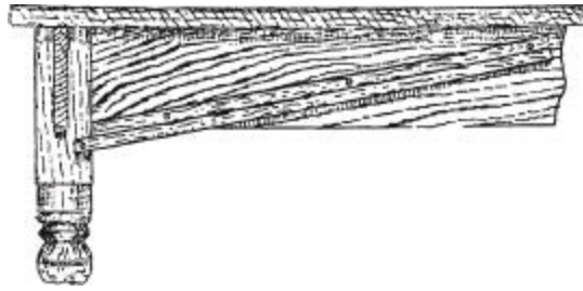
Fig. 1951.—Section of Table showing Drawer Runners.
