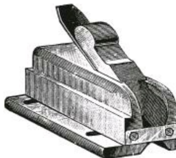
Fig. 177.—Preston's Chamfer Plane with Adjustable Fence.
