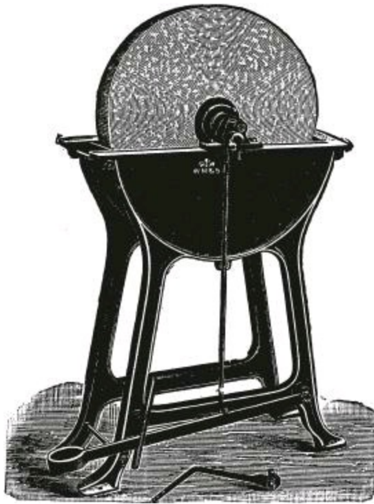
Fig. 435.—Treadle Grindstone on Iron Stand.
