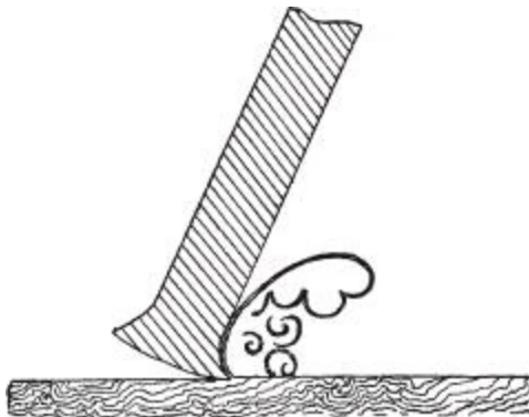
Fig. 414.—Diagram showing Action of Scraper.
