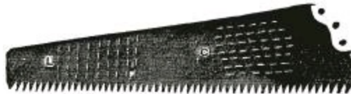
Fig. 317.—Hand saw Buckled Lengthways.
