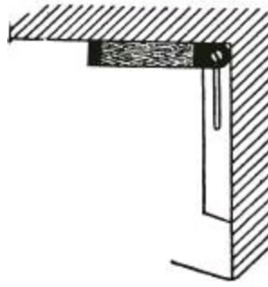
Fig. 818.—Obtaining Angle for Cutting Shelf.
