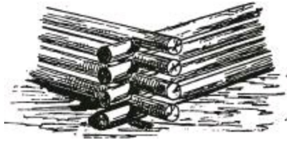
Fig. 1447.—Notched Logs forming Hut Walls.
