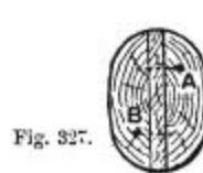
Figs. 326 and 327.—Fastening on Hammer Head with. Nailed Wedge.
