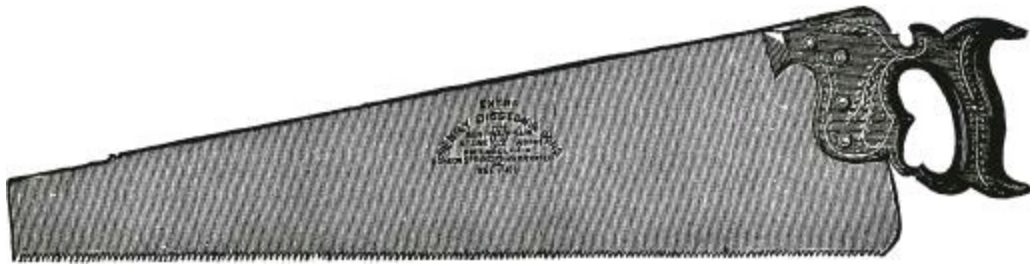
Fig. 239.—Hand Saw with Nibbed Back.
