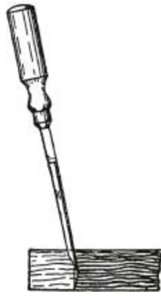
Fig. 674.—Undercutting in Dovetailing.
