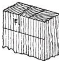
Fig. 680.—Saw Kerf in Waste Portion.
