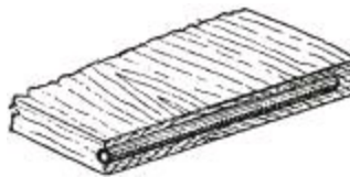
Fig. 2117.—Metal Tubing in Mantelboard.
