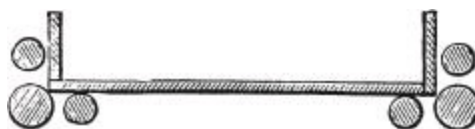
Fig. 1668.—Plan showing how Door is Hinged.
