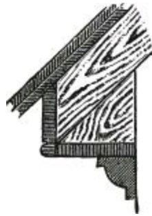
Fig. 1334.—Section of End of Roof Rafters.
