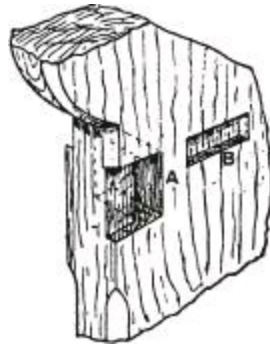
Fig. 1362.—Housings in Seat End.
