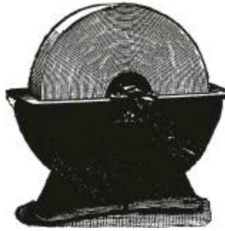
Fig. 434.—Grindstone in Dwarf Iron Stand.
