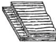
Fig. 770.—Half-lap for Knife-box Corners.
