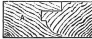
Fig. 209.—Two Pieces of Wood Scribed Together.
