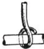
Fig. 1527.—End of Suspending Rod with Tie-rod.
