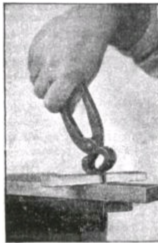
Fig. 470.—Withdrawing Nail with Pincers.
