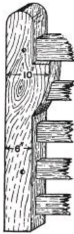
Fig. 1257.—Trussed Harr of Field Gate.
