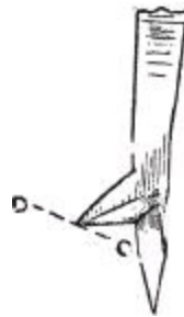
Fig. 393.—Faulty Centre Bit Router.
