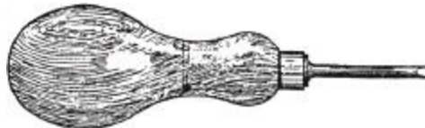
Fig. 364.—Bradawl with Fixed Blade.
