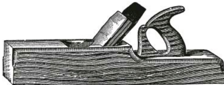
Fig. 156.—Sunk Handle Jack Plane with Closed Toat.
