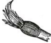
Fig. 492.—Glue Brush with Bent Hair.
