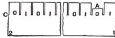
Fig. 696.—Gauge for Marking Box Pin Joint.
