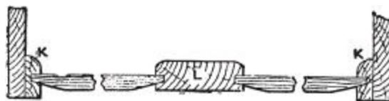
Fig. 2231.--Section through Drawer.
