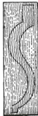
Fig. 2369.—Marking out Cabriole Leg.
