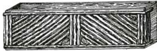
Fig. 1186.—Window Box with Rustic Split Rods.
