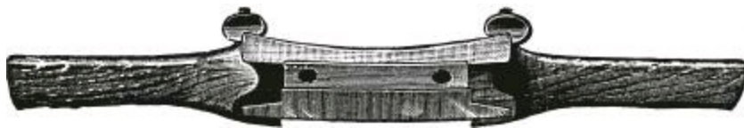
Fig. 153.—Spokeshave with Regulatable Blade.
