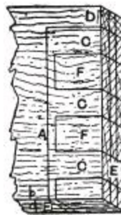
Fig. 650.—Setting Out Plain Clamping.
