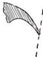
Fig. 394.— Badly Sharpened Nicker.
