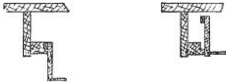
Figs. 1954 and 1955.—Sections of Drawer and Runner.
