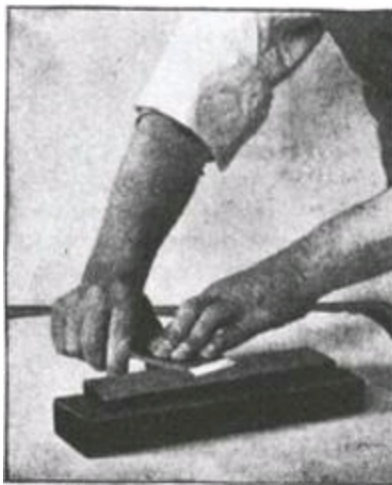
Fig. 197.—Finishing Plane Iron on Oilstone.
