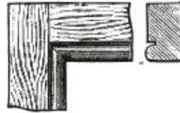
Fig. 74.—Moulding with Mitred Joint.
