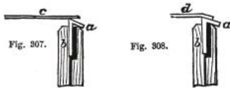
Fig. 307 and 308.—Hammer-setting Teeth on Plate.
