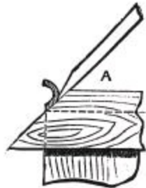
Fig. 76.—Using Chisel with Mitre Template.
