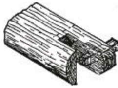
Fig. 1361.—Tenon on Front Rail of «eat.
