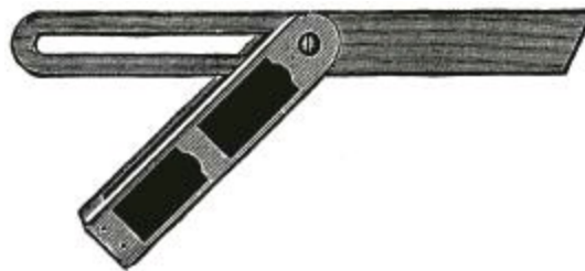
Fig. 18.—Brass Frame Sliding Bevel.
