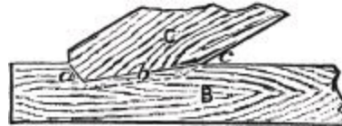
Fig. 630.—Oblique Mortise and Tenon Joint for Rafter and Tie-beam.
