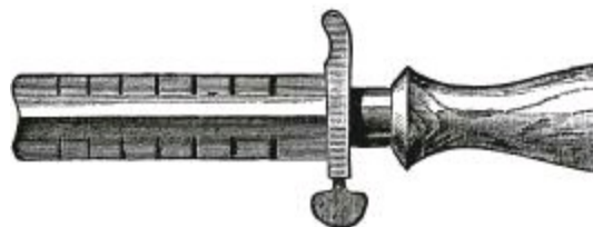
Fig. 297.—Saw-set with Gauge.
