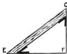
Fig. 1337.—Setting out Hip Rafters.
