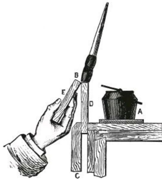
Fig 547.—Gluing Butt Joint, Side View.
