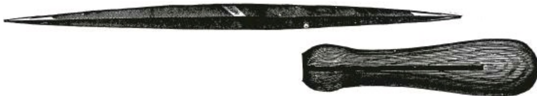
Fig. 277.—Double-ended Saw File and Handle.
