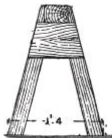
Fig. 102.—End Elevation of Sawing Stool.
