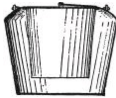
Fig. 481.—Section through Glue-pot.
