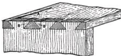
Fig. 669.—Marking Dovetails with Tenon Saw.
