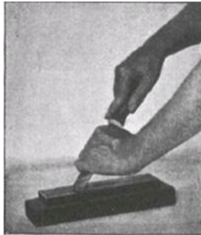
Fig. 146.—Sharpening Chisel on Oilstone.
