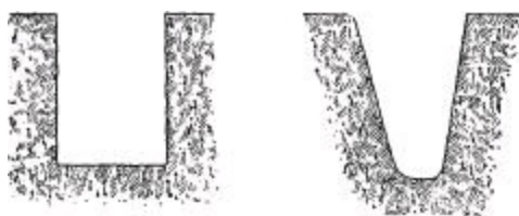
Figs. 1288 and 1289.—Section of Post-hole Properly and Improperly Dug.
