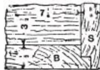
Fig. 774.—Joint of Sides and Bottom of Box.
