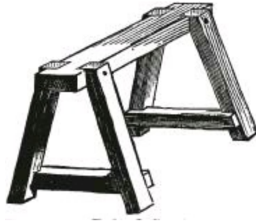
Fig. 105.—Bolted Sawing Stool.
