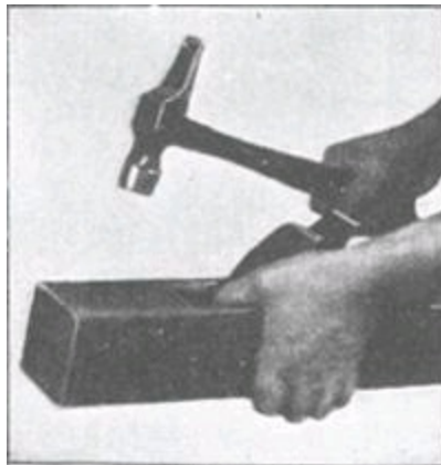
Fig. 158.—Knocking out Iron of Jack Plane.
