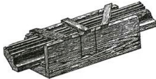
Fig. 60.—Mitre Box with Strengthening Pieces.
