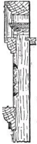
Fig. 2319.—Vertical Section through Pediment.
