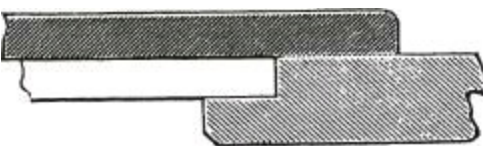
Fig. 2289.—Square-edged Silvered Glass in Shallow Rebate.
