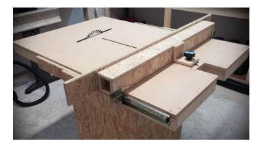
Step 1: Firstly, I cut these pieces for the fence, which are made of OSB.
