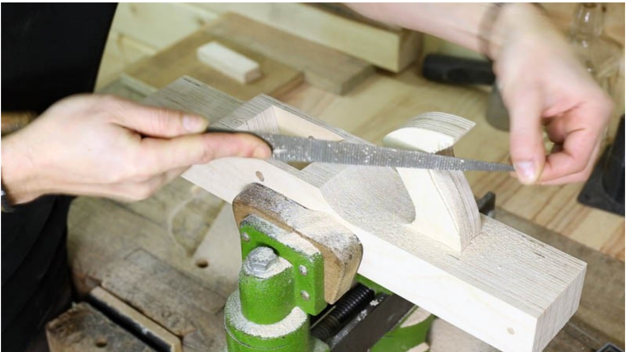
Give the handle its final ergonomic shape to make it fit comfortably in your hand.
