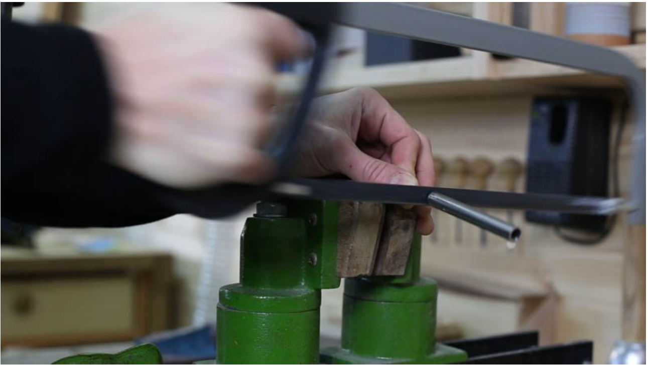
Now we can cut the steel pipe.
