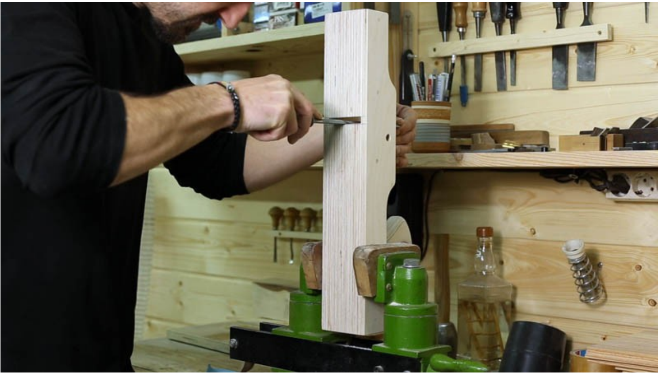
Here you can use a rasp to square the blade hole
