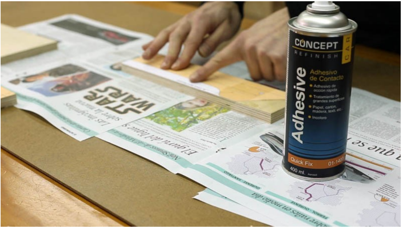
Glue all the templates to the hard plywood using spray adhesive
