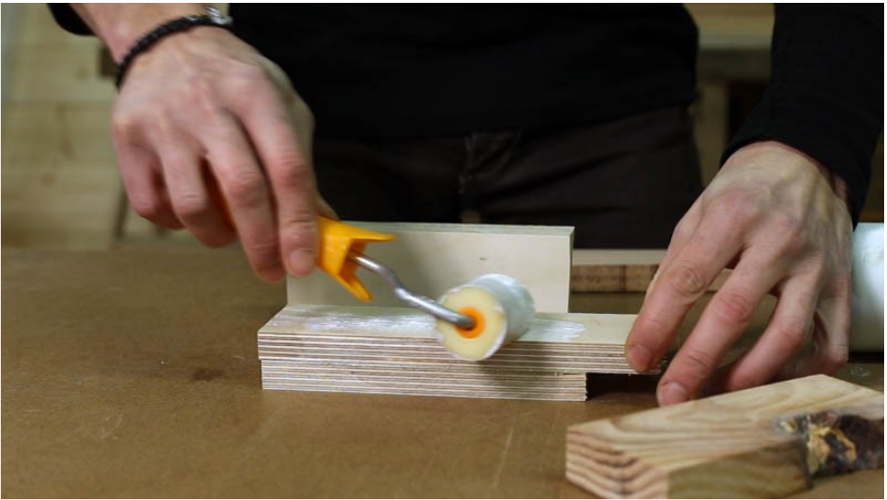
Glue four pieces of plywood to build the wedge
