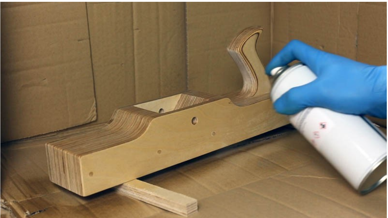
At this point, the varnish can already be applied. I used two coats of nitrocellulose spray lacquer.
