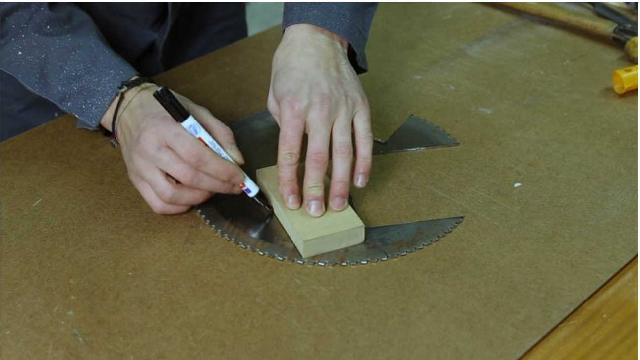
To make the blade you can recycle an old cutting disc from an circular saw. You can use a wood template of the same size to mark the disc before cutting.
