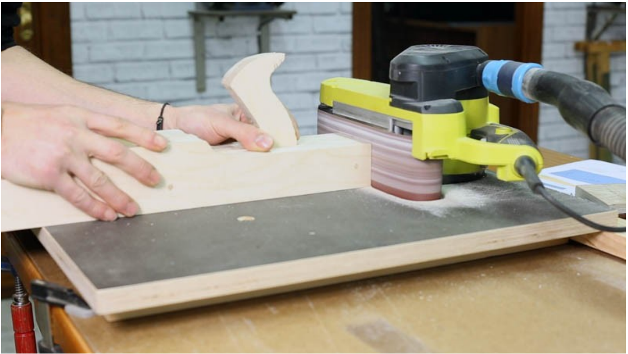
Once the glue is dry and we can start sanding.
