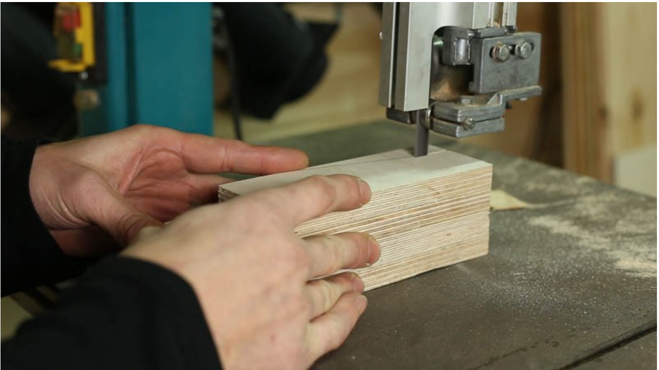
Once it is dry, mark it and cut it on the band saw.
