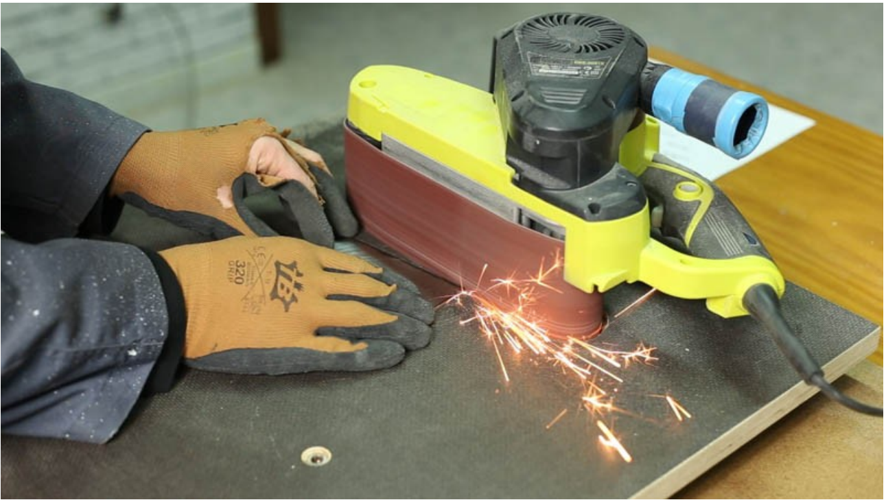
Sand it with the belt sander making sure it remains squared.
