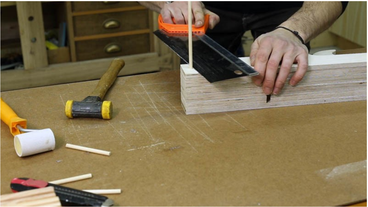
Put the dowells in place and cut them.
